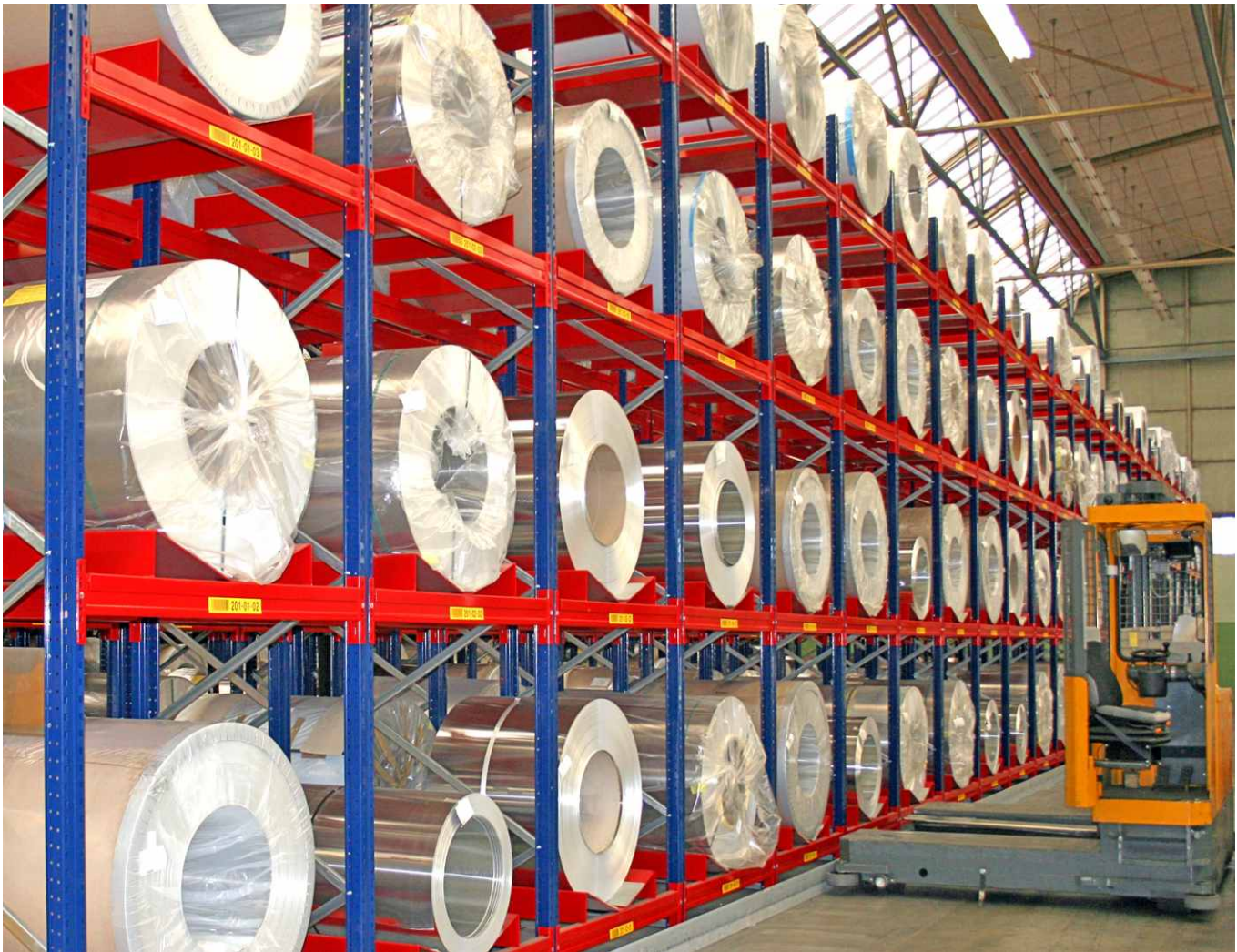
Pallet racking adapted to store coils.
